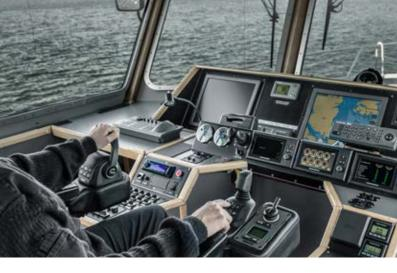
The buttons on the joystick put a unique combination of functions within your easy reach. Dynamic Positioning, Joystick Driving, Joystick Docking and High Mode offer easier handling, increased safety, and reliable operation.
